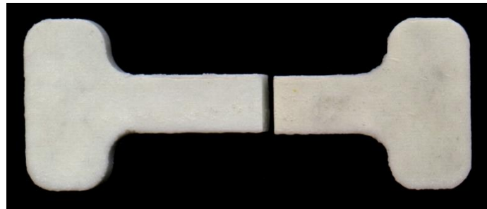
Figure 17. Fractured cement specimen
