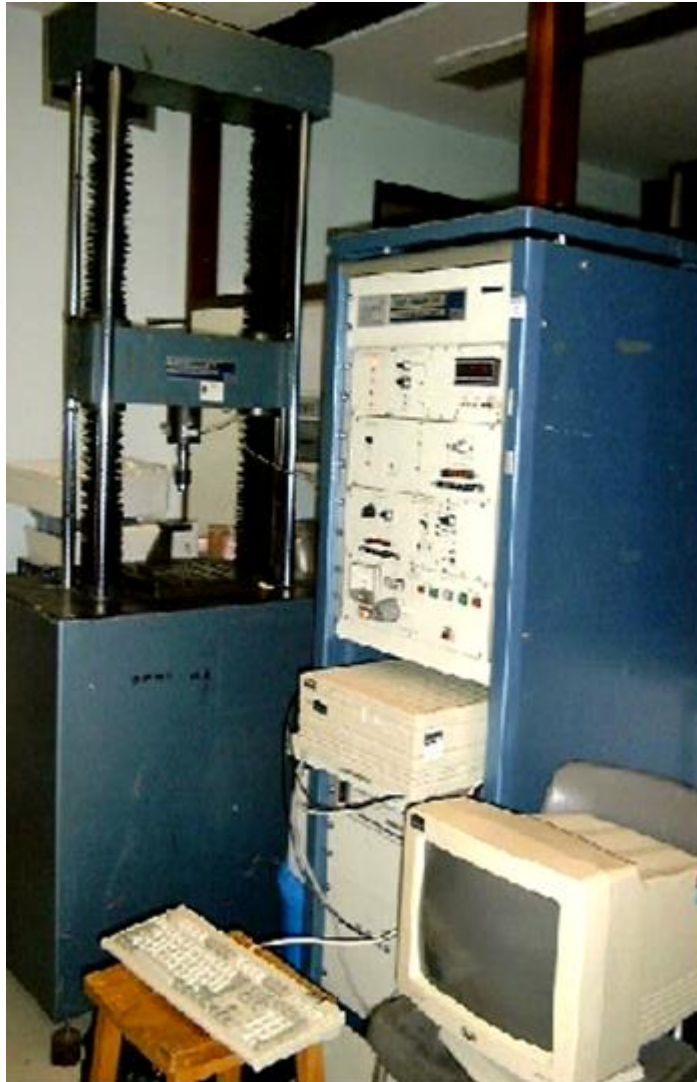
Figure 15. Universal testing machine connected to computer
