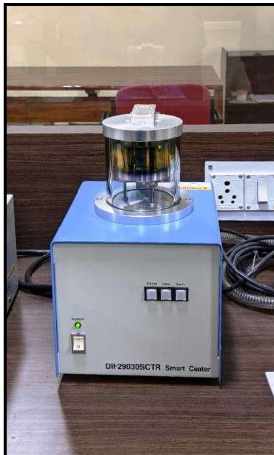
Figure 5: Sputter coating device being used for ion coating of the dentin specimens
