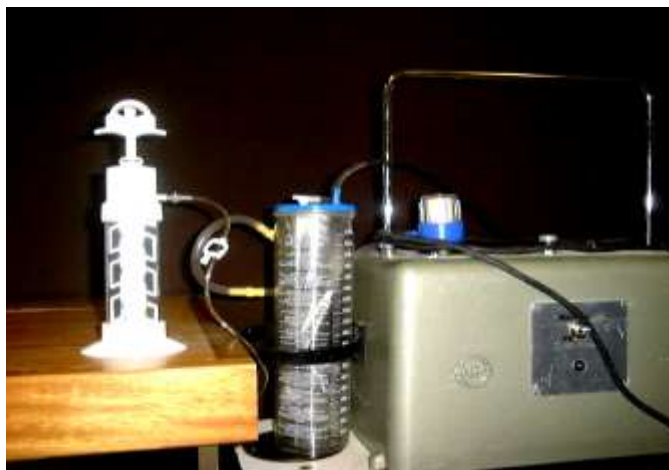
Figure 7. Mixing syringe and vacuum system
