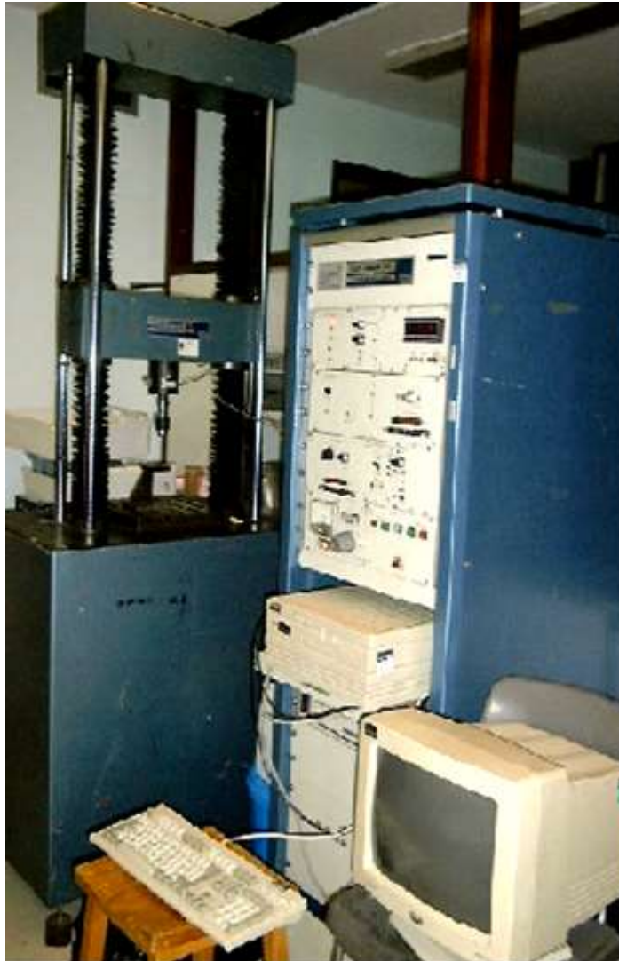
Figure 15. Universal testing machine connected to computer
