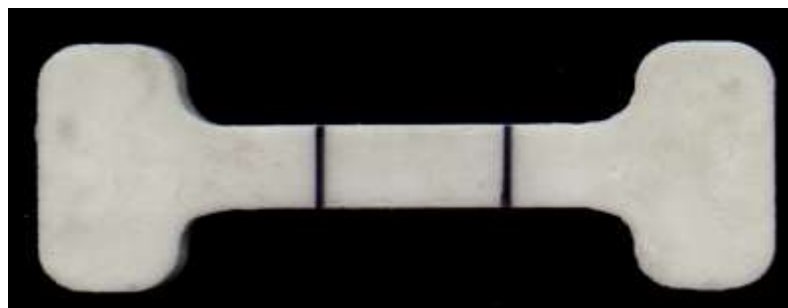
Figure 12. Cement specimen showing the test segment
