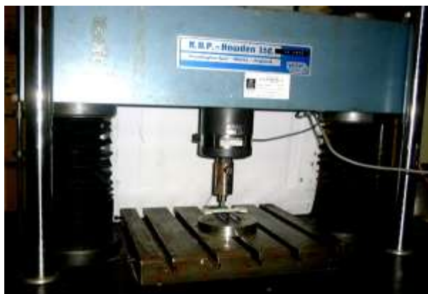
Figure 16. Three-point bending test
