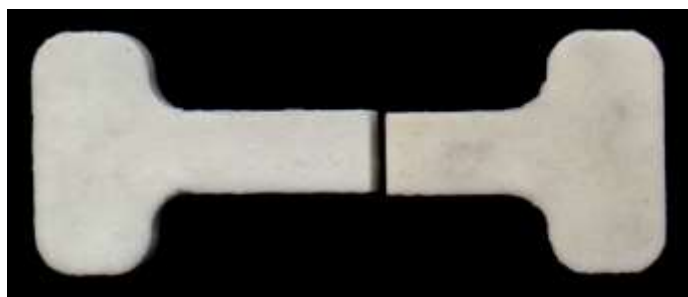
Figure 17. Fractured cement specimen
