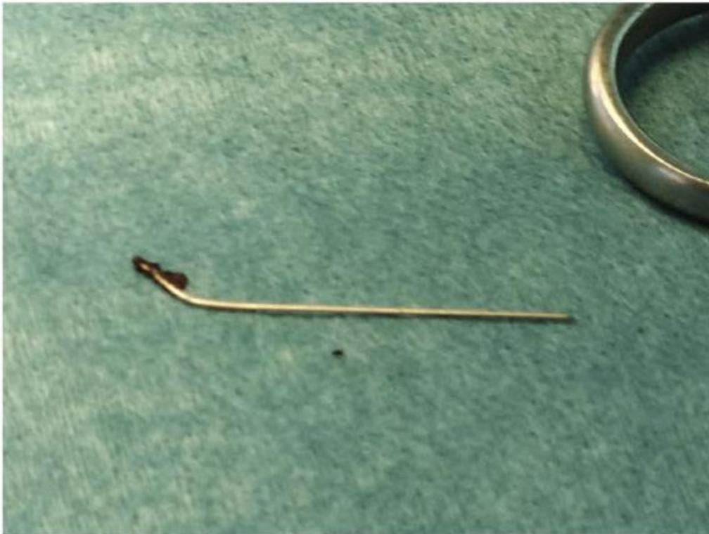
**Figure 3.** Broken fragment of the needle
