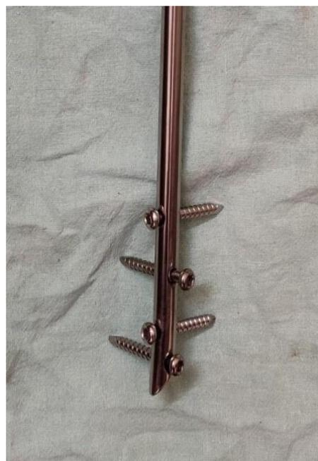
**Figure 2** – ETNS with 4 distal locking holes
