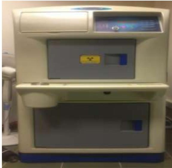
**Figure 17:** Gammacell Irradiator
