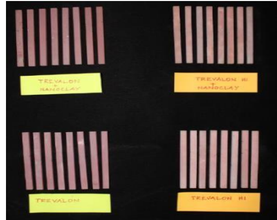
Fig 6. Samples for testing Impact strength
