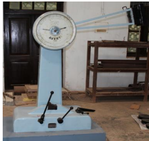
Fig 8. Charpys Impact Testing Machine
