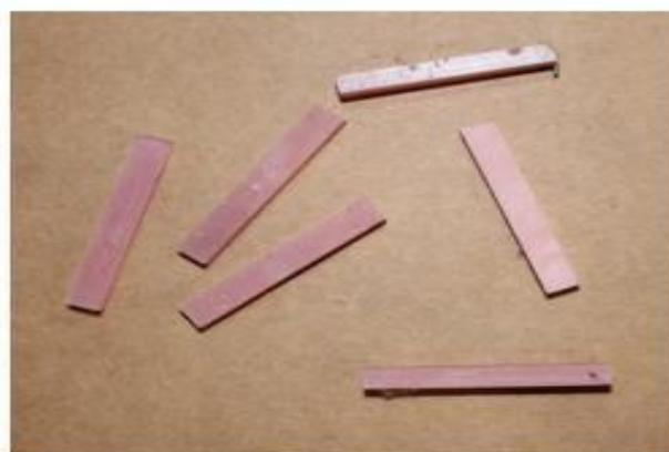
Fig 10. Broken Samples after impact strength testing
